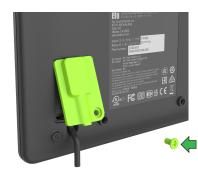
Install the cable cover by installing the top side first and rotating it down. Secure the door with the M3 screw included.
