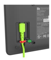
Connect the micro USB cable. Ensure the rubber gasket (red) is all the way inside the cable cover area.
