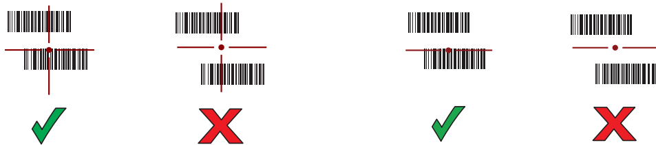
Figure 21 Pick List Mode with Multiple Barcodes in Aiming Pattern: Standard and Extended Range
