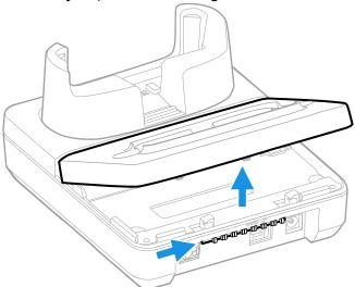
3. Release the latch and lift the old cup out of the base.
