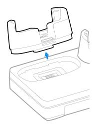
4. Insert the new cup tilted slightly towards the front of the base.
