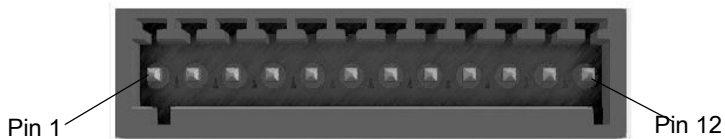
Figure 161 FX9600 RFID Reader GPIO Connection
