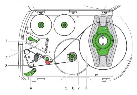
Figure 19 Guidance of the material in peel-off mode
