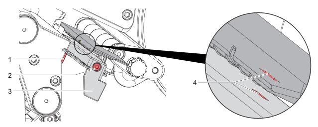
Figure 28 Cleaning the label sensor
