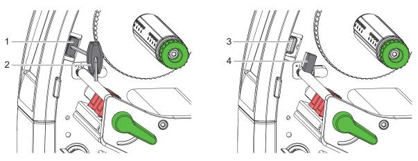
Figure 8 Installing the Wi-Fi stick
