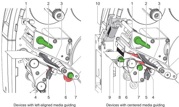
Inserting the media into the printhead
