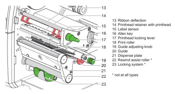
Figure 3 Print unit - devices with left-aligned media guiding (excepting SQUIX 8.3)
