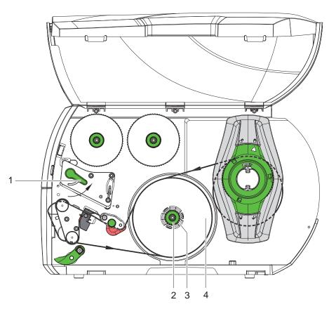
Figure 18 Removing the wound roll
