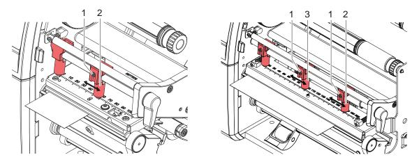
Figure 22 Setting the head locking system - devices with left-aligned media guiding
