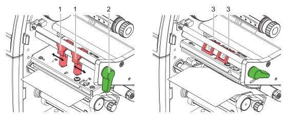
Figure 23 Setting the head locking system - devices with centered media guiding
