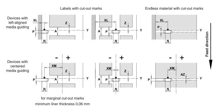
Figure 33 Cut-out mark dimensions
