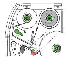
Figure 26 Transfer ribbon feed path
