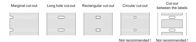
Figure 34 Samples for cut-out marks
