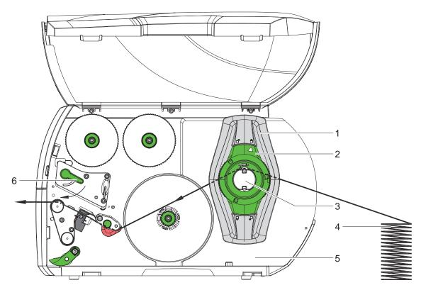
Figure 21 Feed path of fanfold media
