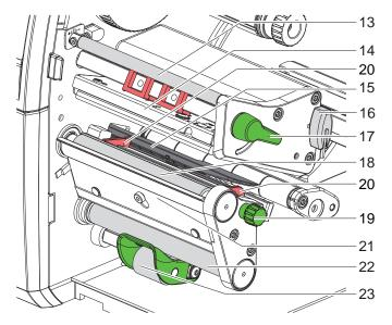
Figure 5 Print unit - devices with centered media guiding
