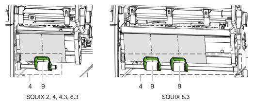
Figure 20 Aligning the pinch rollers
