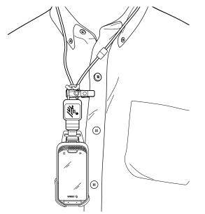
To adjust the length of the lanyard, press and hold the adjustment button and slide the button up or down the string.
