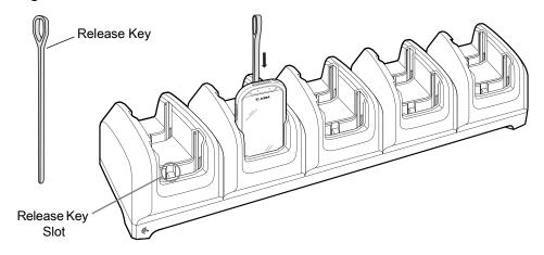
Figure 25 Manual Release of the EC30
