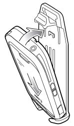
4. Use the clip to secure the retractable lanyard to clothing.
