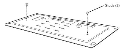
2. Align and install 10-Slot cradle onto studs of plate.
