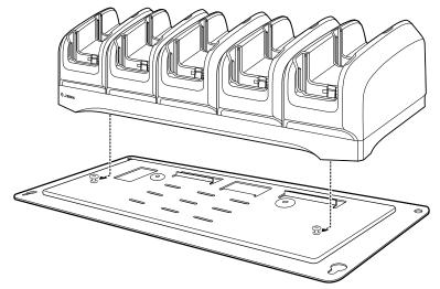
3. Secure cradle to the top tray with two M2.5 safety screws.
