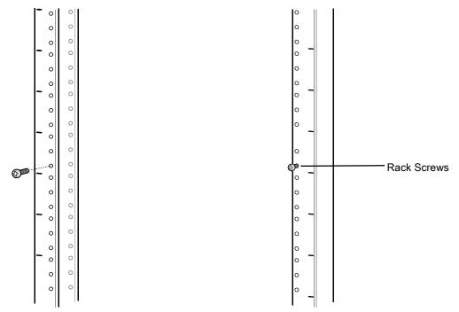
**11.** Align the mounting plate's top mounting key holes with the screws.
