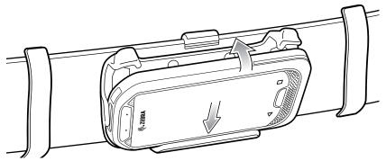
3. Rotate the device for the best viewing angle.
