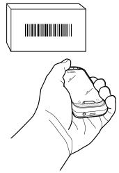
3. Press and hold the scan button. The white aiming pattern turns on to assist in aiming.
