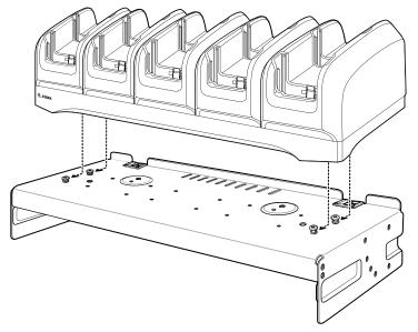
8. Secure cradle to the top tray with two M2.5 safety screws.
