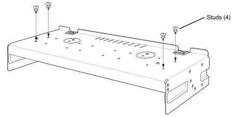
7. Align and install 10-Slot cradle onto studs of the top tray.
