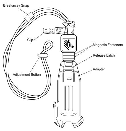
1. Snap the end of the lanyard onto the adapter.
