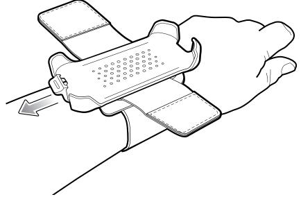
3. Tighten the strap and press the hook and loop material together.
