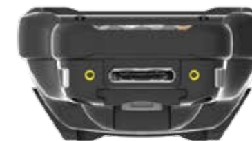
No I/O Cover installed
