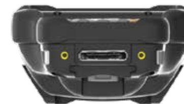
No I/O Cover installed
