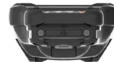
I/O Cover installed
