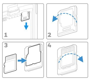
**Note:** Always power off the computer before attempting to install or remove a microSD card.
