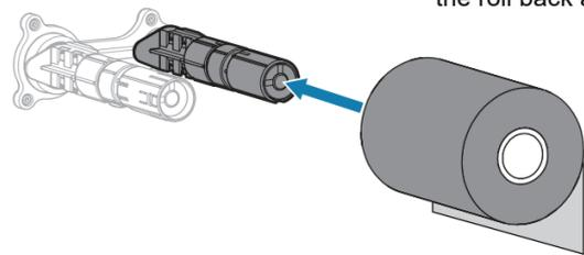
Place an empty core on the ribbon take-up spindle as shown. Push the core back as far as it will go.
