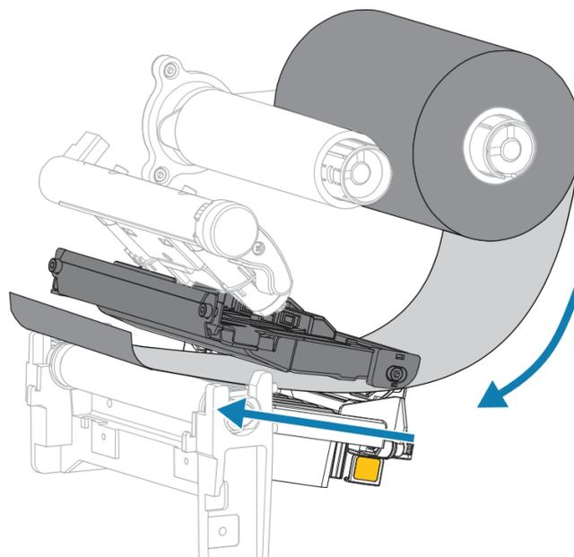
Wrap the ribbon around the core several times, and then rotate the spindle to tighten and align the ribbon.
