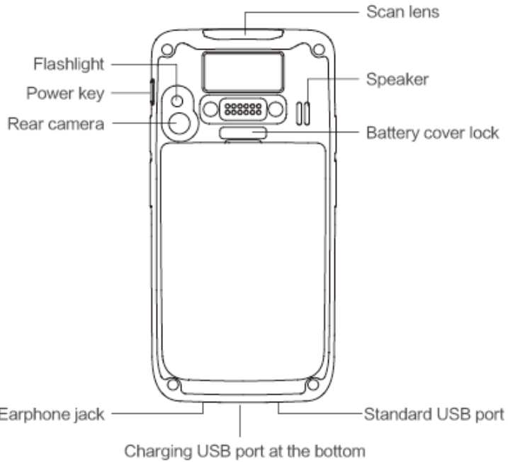
FIGURE 1-2 REAR VIEW OF NAUTIZ X2
