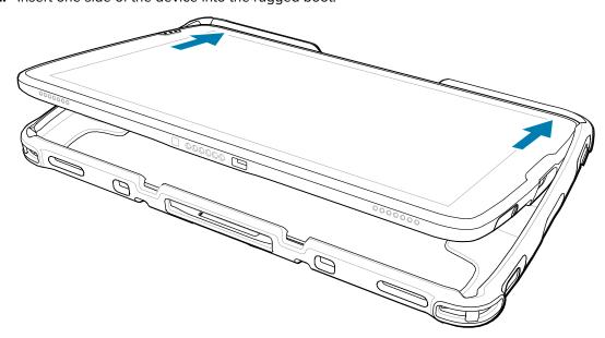
**2.** Push the other side of the device into the rugged boot.
