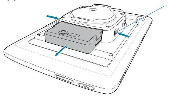
**3.** Remove dummy battery insert.
