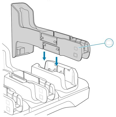
**2.** To charge a tablet with the rugged boot, hold the insert so that the rugged boot icon is on top.
