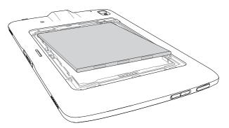
**10.** Gently push the battery towards the contacts (1) while rotating the battery down into the battery well (2), ensuring it is seated properly.
