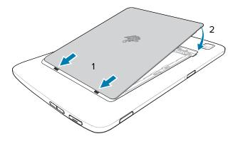
**13.** Carefully press down around the edges of the cover. Make sure that the cover is seated properly.
