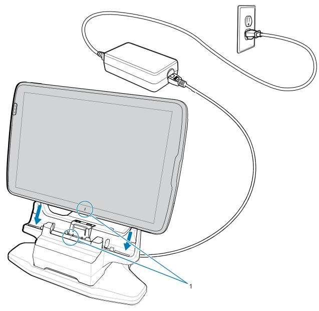
2. Insert the device into the cradle (1) and rotate it backwards (2) until it clicks.
