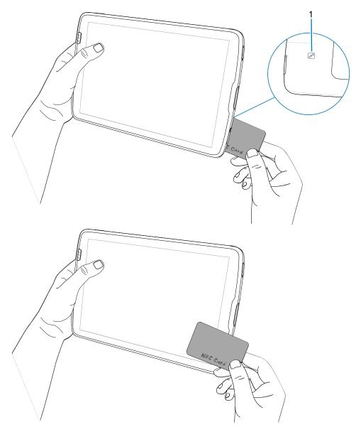
The tablet can read NFC cards from the front or back of the device.
