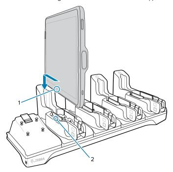
**4.** Place the device down into the slot with the display facing towards the Battery Charger.
