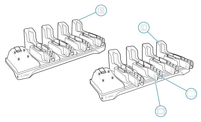
**1.** To charge a tablet without the rugged boot, hold the insert so that the tablet icon  $\square$  is on top.
