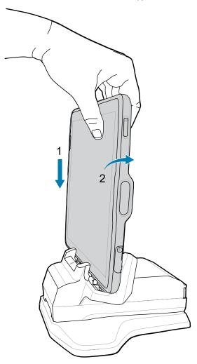
The device is locked in the cradle and the device Charging LED indicates charging.
