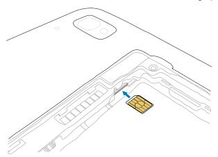
**8.** Push the SIM card in and ensure that it locks into place.
