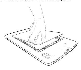
**2.** Insert the tabbed end of the expansion back into the battery well (1). Ensure that the tabs on the expansion back are aligned with the slots in the battery well.
