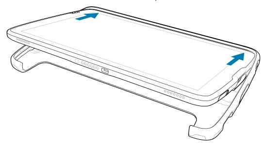
2. Push the device into the open side of the handstrap.
