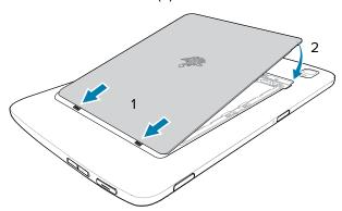
**5.** Carefully press down around the edges of the cover. Make sure that the cover is seated properly.
